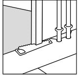
The last and first row of planks should be at least 8 cm wide. We recommend measuring and cutting the first rows first and laying them dry. Cut wooden frames to plank height and lay the floor covering under the frames. For steel frames, lay the dryback covering with a minimum joint of at least the same material thickness and seal the joint with a suitable natural stone silicone.
