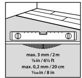
For the installation of dryback flooring, it is standard practice to apply a 2.0 to 3.0 mm thick layer of levelling compound with the spreader, followed by smoothing the surface with a spiked roller. Any remaining unevenness on the levelled floor must be removed after drying with a finishing spatula or a disc floor machine, followed by vacuuming the surface thoroughly.
